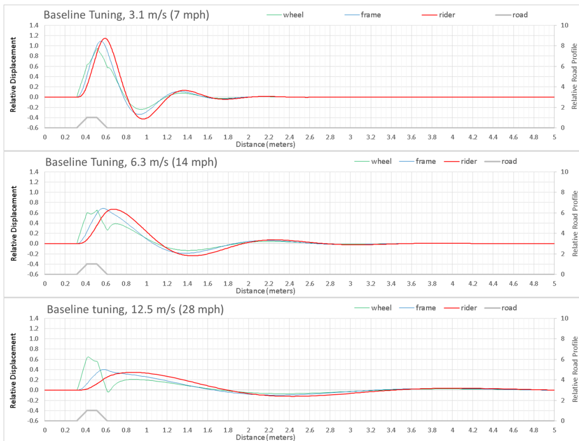
Figure 9 –Transient response. The bicycle is ridden from left to right. The elevation of the road profile (projected to the secondary axis on the right) is scaled such that the dimension b of the raised block specified in Figure 8 defines the unit of elevation. The red trace (projected onto the primary axis on the left) is the ratio between the vertical displacement of the rider’s body from its static height above the ground and the overall height (dimension b ) of the block. The green and blue traces represent the same quantity for the wheel and frame, respectively.
